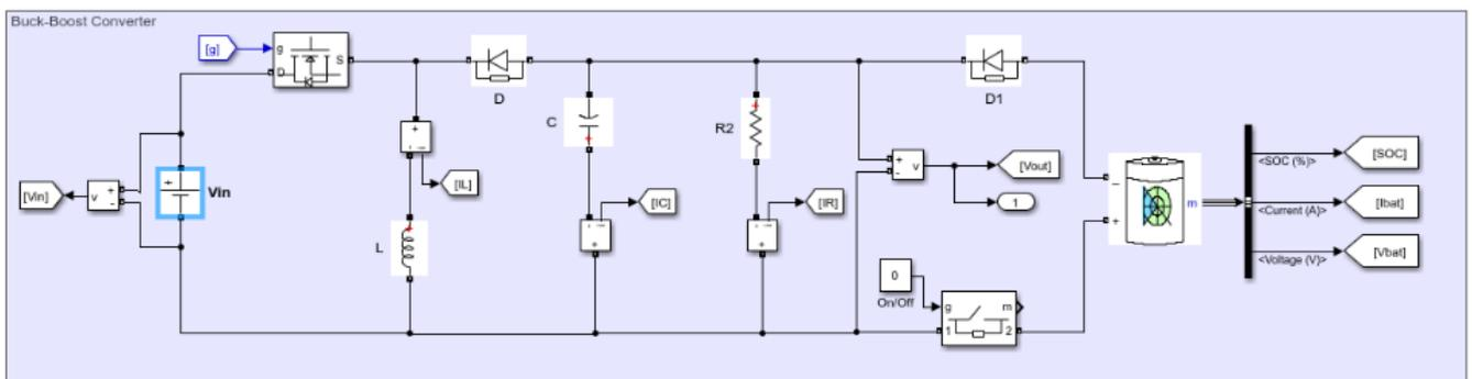
Fig. 2: MATLAB/Simulink model of DC/DC Buck-Boost
